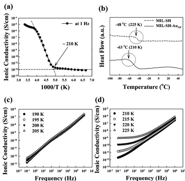
**Fig. 3** (a) Temperature-dependent ionic conductivity of 72 wt% MIL-SH- $\text{Au}_{\text{NPs}}$  measured at a fixed frequency of 1 Hz. (b) DSC analysis of pure MIL-SH and 72 wt% MIL-SH- $\text{Au}_{\text{NPs}}$ . Frequency-dependent ionic conductivity of 72 wt% MIL-SH- $\text{Au}_{\text{NPs}}$  at temperatures (c) below and (d) above the glass transition temperature ( $T_g$ ).
