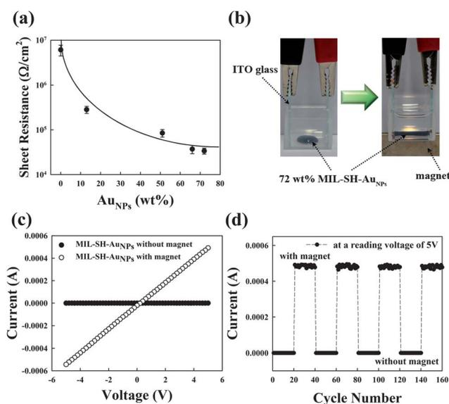
**Fig. 4** (a) The measured sheet resistance of MIL-SH- $\text{Au}_{\text{NPs}}$  as a function of the  $\text{Au}_{\text{NP}}$  concentration using the four-point probe method. (b) The digital images show the magnetic response of the 72 wt% MIL-SH- $\text{Au}_{\text{NP}}$  fluids between two ITO electrodes to an external magnet. (c)  $I$ - $V$  curves and (d) cycling tests of MIL-SH and 72 wt% MIL-SH- $\text{Au}_{\text{NP}}$  fluids under the effects of an external magnet.
