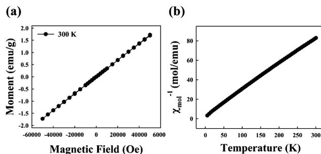
**Fig. 2** (a) Magnetization of 72 wt% MIL-SH-AuNP as a function of the external magnetic field measured at 300 K. (b) The reciprocal molar susceptibility curve of 72 wt% MIL-SH-AuNP obtained to confirm the paramagnetic properties of the fluid.
