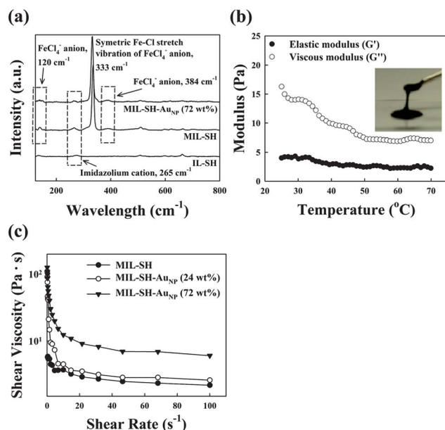
**Fig. 1** (a) Raman spectra of IL-SH, MIL-SH and MIL-SH-AuNP obtained to confirm the presence of FeCl<sub>4</sub><sup>-</sup> anions. (b) Elastic and viscous moduli as a function of temperature for 72 wt% MIL-SH-AuNP (*i.e.*, AuNP concentration of 72 wt%). The inset demonstrates the fluidic behavior of MIL-SH-AuNP (72 wt%). (c) Shear viscosity of MIL-SH and MIL-SH-AuNP as a function of shear rate.
