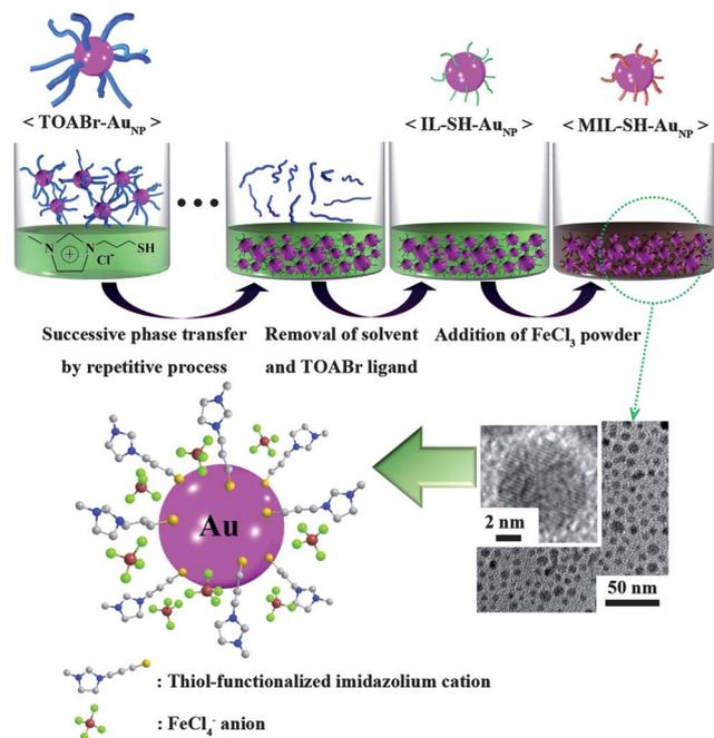
**Scheme 1** Schematics illustrating the preparation of solvent-free MIL-SH and MIL-SH-AuNP.
