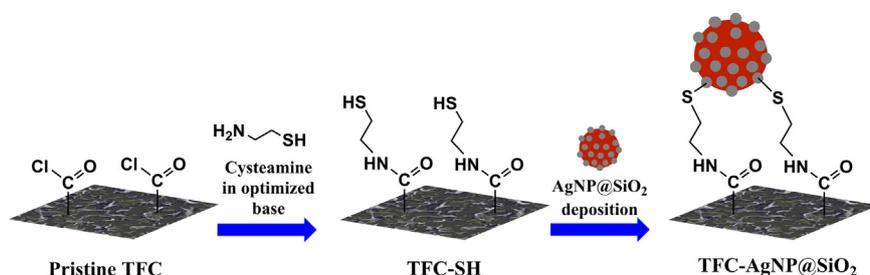
Fig. 2. Schematic illustration of the immobilization of AgNP@SiO<sub>2</sub> particles on a PA TFC membrane.
