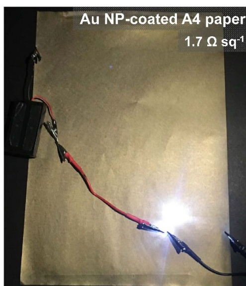
Figure S17. Photographic images of (a) a bare A4 paper (29.7cm x 21.0cm) and a (DETA/TOABr-Au NP) 10 multilayer-coated (29.7cm x 21.0cm) A4 paper and (b) a LED connected through the (DETA/TOABr-Au NP) 10 multilayer-coated A4 paper.
