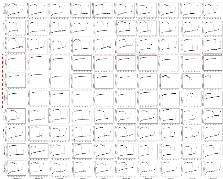
Figure S2. Electrical switching behavior of sol-gel derived Nb 2 O 5 devices measured from 100 samples. About 30 samples within red lines displayed malfunctioning switching behavior. As a result, our devices showed the output performance of about 70 %.
