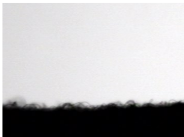
Fig. S8 Water contact angles of the C-CT, carbon paper, and carbon cloth. These results imply that the C-CT has a more advantageous hydrophilic property for electrolyte infiltration than commercial carbon paper and carbon cloth.
