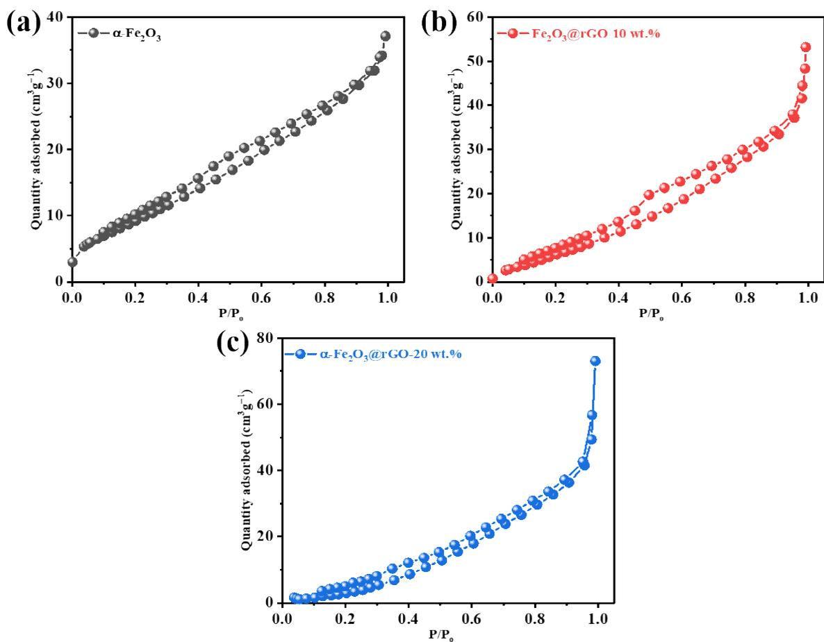
**Figure. S2** BET surface area plots of (a)  $\alpha\text{-Fe}_2\text{O}_3$ , and (b & c)  $\alpha\text{-Fe}_2\text{O}_3@\text{rGO}$  core@shell nanocubes.
