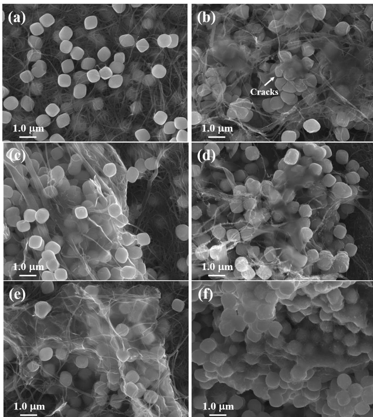
**Figure. S4** FE-SEM images of (a)  $\alpha$ - $\text{Fe}_2\text{O}_3$ /SWCNT, (c)  $\alpha$ - $\text{Fe}_2\text{O}_3$ @rGO-10 wt.%/SWCNT, (e)  $\alpha$ - $\text{Fe}_2\text{O}_3$ @rGO-20 wt.%/SWCNT samples before, and (b)  $\alpha$ - $\text{Fe}_2\text{O}_3$ /SWCNT, (d)  $\alpha$ - $\text{Fe}_2\text{O}_3$ @rGO-10 wt.%/SWCNT and (f)  $\alpha$ - $\text{Fe}_2\text{O}_3$ @rGO-20 wt.%/SWCNT samples after 20 cycles at 0.1 C-rate.
