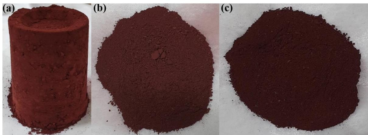
**Figure. S1** Digital images of (a)  $\alpha$ -Fe<sub>2</sub>O<sub>3</sub>, (b)  $\alpha$ -Fe<sub>2</sub>O<sub>3</sub>@rGO-10 wt.%, and (c)  $\alpha$ -Fe<sub>2</sub>O<sub>3</sub>@rGO-20 wt.% powder samples.
