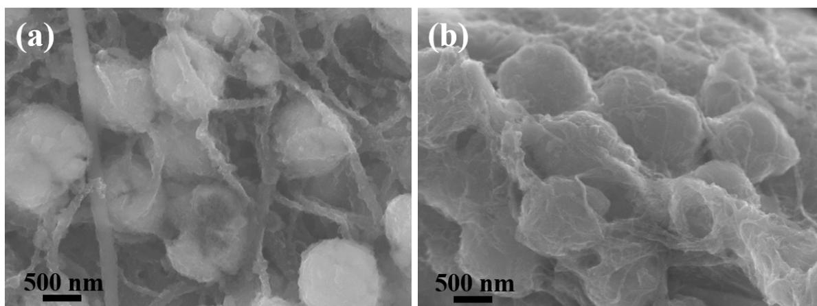
**Figure. S11** FE-SEM images of (a)  $\alpha$ -Fe<sub>2</sub>O<sub>3</sub>@rGO-10 wt.%, and (b)  $\alpha$ -Fe<sub>2</sub>O<sub>3</sub>@rGO-20 wt.% core@shell nanocubes after the 650<sup>th</sup> cycle.
