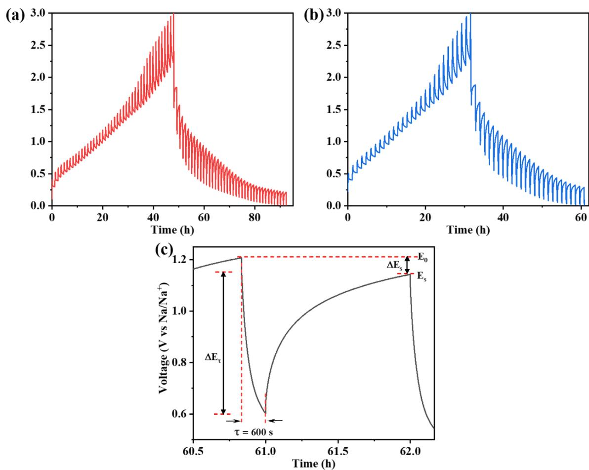
**Figure. S10** GITT plots of (a)  $\alpha\text{-Fe}_2\text{O}_3$ , and (b)  $\alpha\text{-Fe}_2\text{O}_3$ @rGO-20 wt.% samples, and (c) single titration curve of  $\alpha\text{-Fe}_2\text{O}_3$ @rGO-10 wt.% sample during the discharge.
