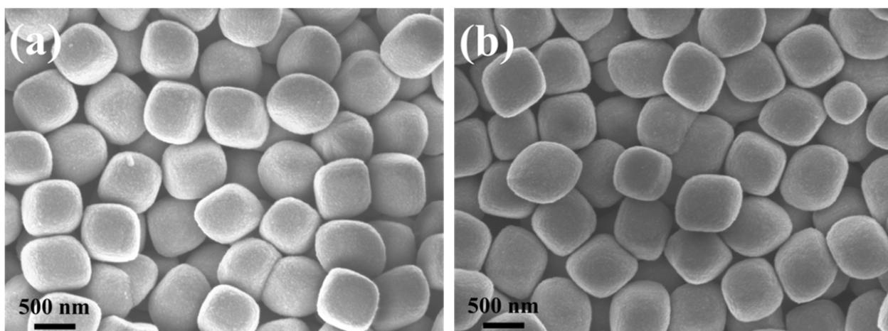
**Figure. S3** FE-SEM images (a)  $\alpha$ -Fe<sub>2</sub>O<sub>3</sub>, and (b) PEI- $\alpha$ -Fe<sub>2</sub>O<sub>3</sub> nanocubes.
