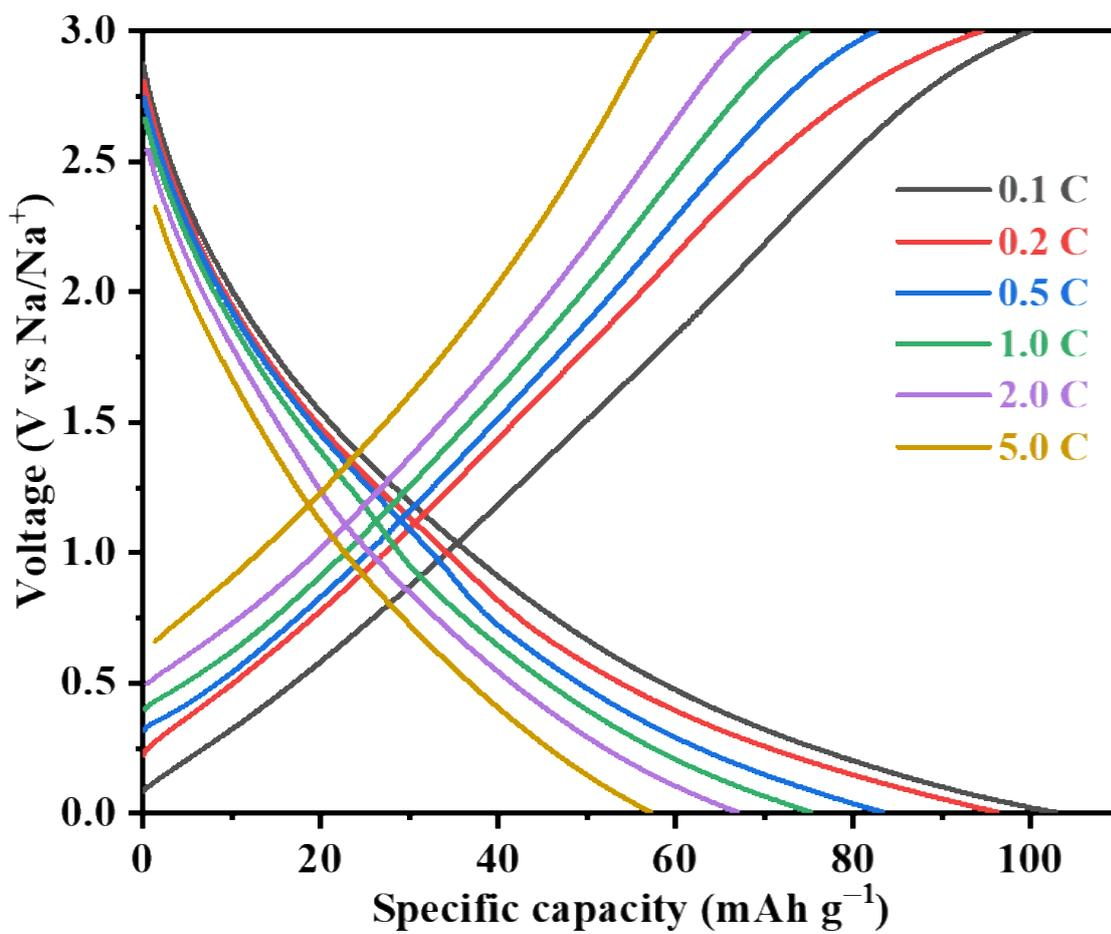
**Figure. S9** GCD plot of SWCNTs electrode at various C-rates with an electrode mass of 1.0 mg cm<sup>-2</sup>.
