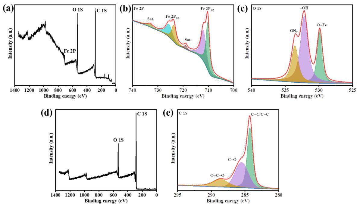
**Figure. S7** (a & d) XPS survey spectrums of  $\alpha$ -Fe<sub>2</sub>O<sub>3</sub> and rGO, and (b & c) high-resolution XPS spectra of Fe2p, and O1s of  $\alpha$ -Fe<sub>2</sub>O<sub>3</sub>, and (e) high-resolution XPS spectra of C1s of rGO.
