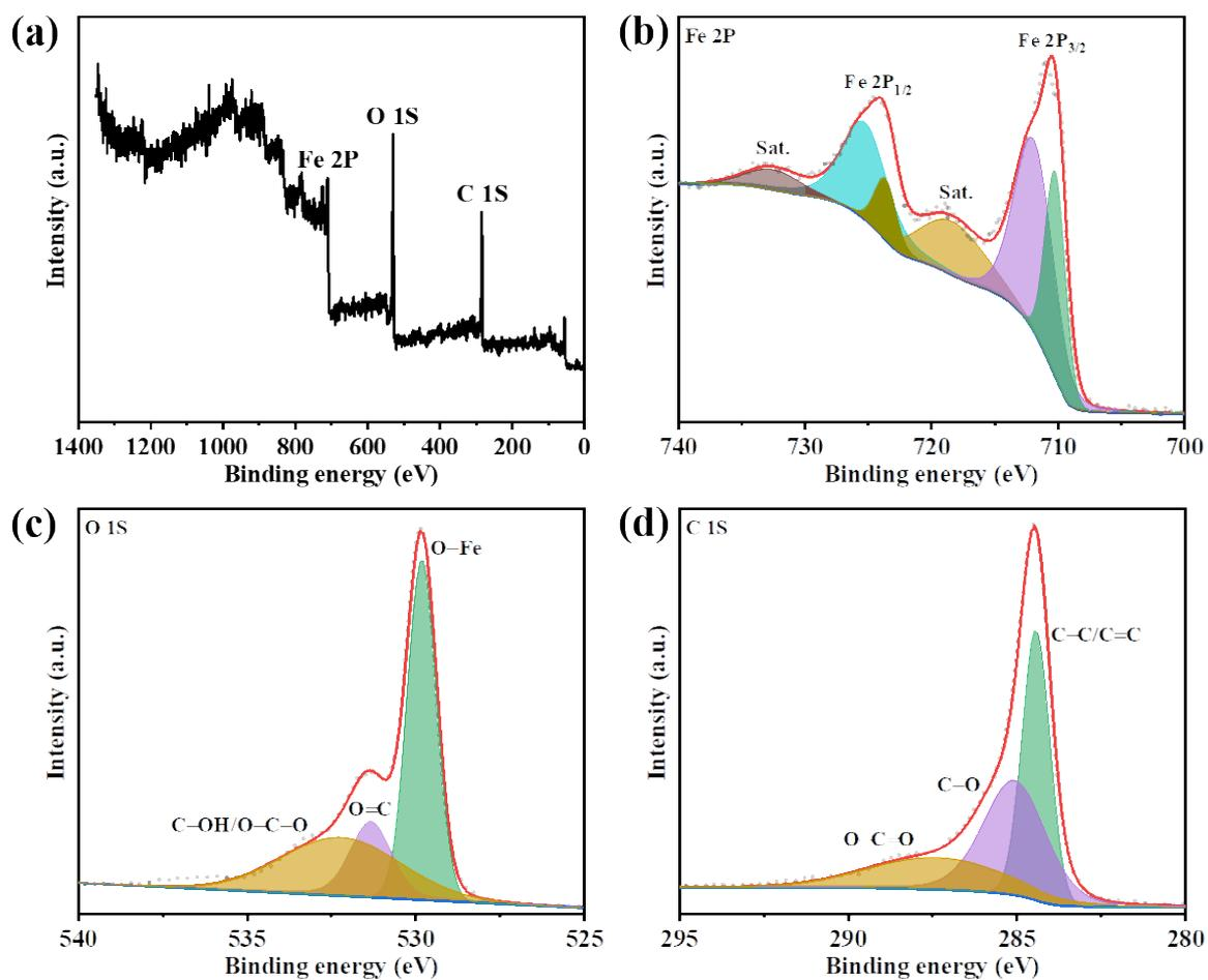
**Figure. S8** (a) XPS survey spectrum, and (b-d) high-resolution XPS spectra of Fe2p, O1s, and C1s of  $\alpha$ -Fe<sub>2</sub>O<sub>3</sub>@rGO-20 wt.% core@shell nanocubes.
