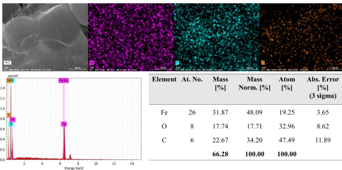
**Figure. S6** SEM-EDS color mapping, and EDS spectra of  $\alpha$ -Fe<sub>2</sub>O<sub>3</sub>@rGO-20 wt.% core@shell nanocubes.
