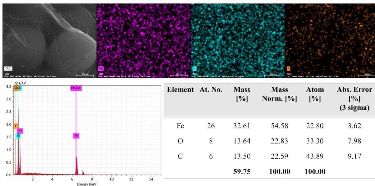
**Figure. S5** SEM-EDS color mapping, and EDS spectra of  $\alpha$ -Fe<sub>2</sub>O<sub>3</sub>@rGO-10 wt.% core@shell nanocubes.
