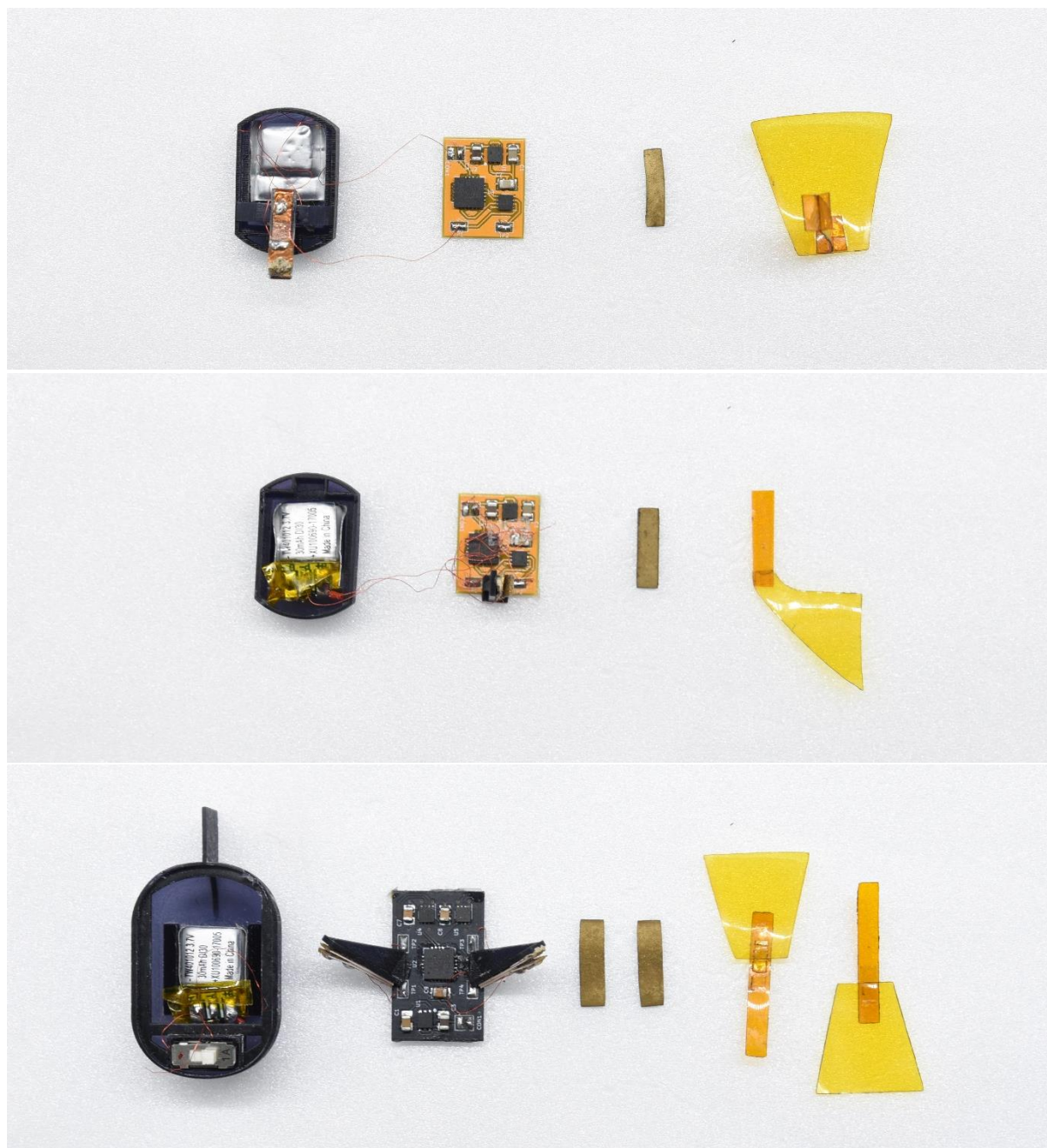
Figure S27. Aquabots with flapping and sculling motions. Photographic images of aquabots composed of robot body, battery, circuit board, fins and WNE-actuators.
