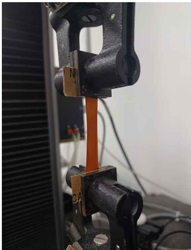
Figure S6. Photographic image of universal testing machine (UTM) measurement of the SPEs.
