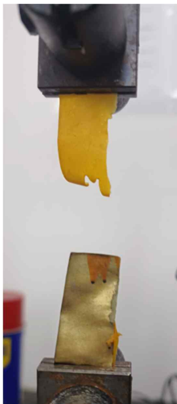
Figure S11. Photographic image of directly coated SPE with UV-crosslinking on lithium metal foil after 180° peel-off test.
