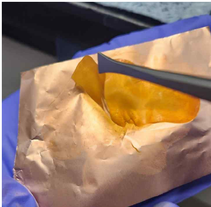
Figure S10. Peel test of the freestanding SPE: It easily separates from the Cu foil, making it impossible to perform a 180° peel-off test.
